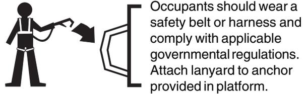
Occupants should wear a safety belt or harness and comply with applicable governmental regulations. Attach lanyard to anchor provided in platform.
